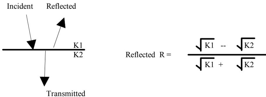
The effect of moisture in the soil is to increase the values of the dielectric coefficients and consequently the difference between K1 and K2. The result is thus a stronger reflection and in this case allowing the soil stratigraphy to be seen. Chart 2. Below shows the rapid change in reflectivity as the difference in dielectric coefficients K1 and K2 is increased.
